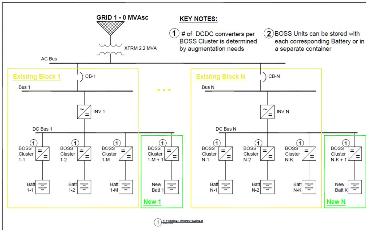
Figure 2: The diagram shows the rack level DC augmentation strategy where a BOSS or some number of BOSS units based on the total current that needs to be managed based on the C rate of the system and electrical specifications of the battery rack.
