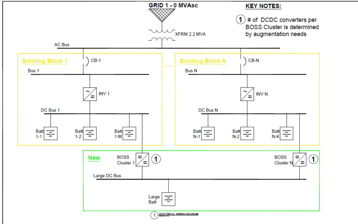
Figure 3: The diagram shows a container level augmentation, where a new BESS container can be installed and have energy delivered to individual containers that need additional storage capacity.
