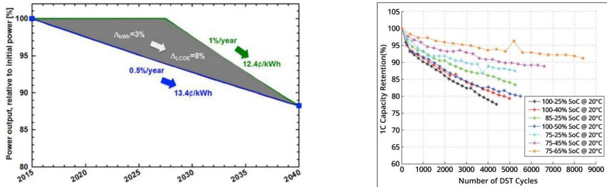
Figure 1: The diagram on the left (source: NREL) shows the typical degradation in generation of a PV plant, while the chart on the right shows the degradation of a typical lithium-ion battery over time based on various cycling scenarios (Source: Battery University)
