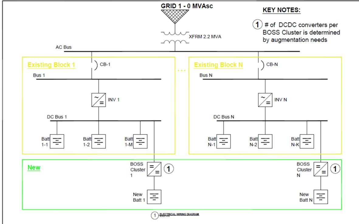
Figure 4: The diagram shows a container/rack level augmentation, where a new BESS container can be installed and have individual racks within the container assigned to different containers on site.
