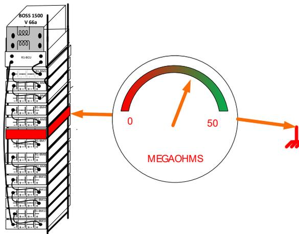
Figure 5: The BOSS' Leak Locator™ identifies the location and severity of a single ground leak.
