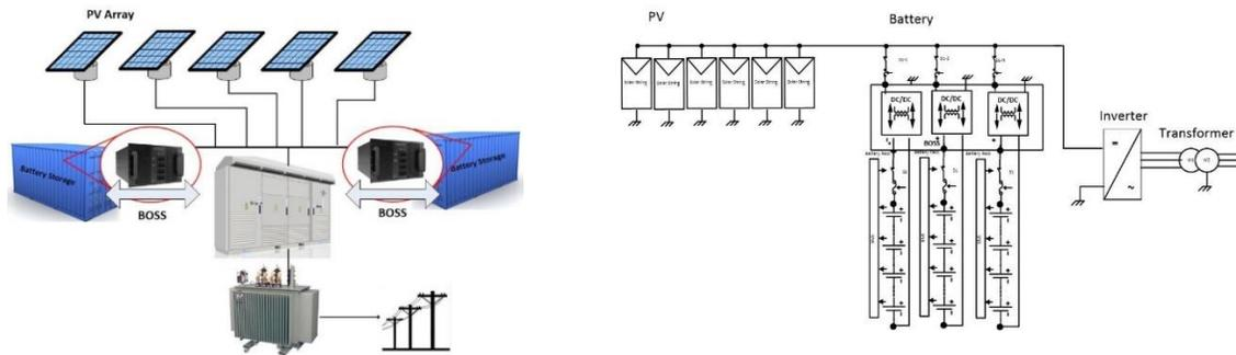
Figure 6: The drawings shown above provide more detailed schematics of a battery centric approach to DC coupling. On the left is an illustration of a BESS wired with bi-directional DC:DC optimizers connected to a DC bus where the DC bus is connected a grid tied inverter that is performing maximum power point tracking in the PV array. The schematic on the right shows how such a system would be wired.
