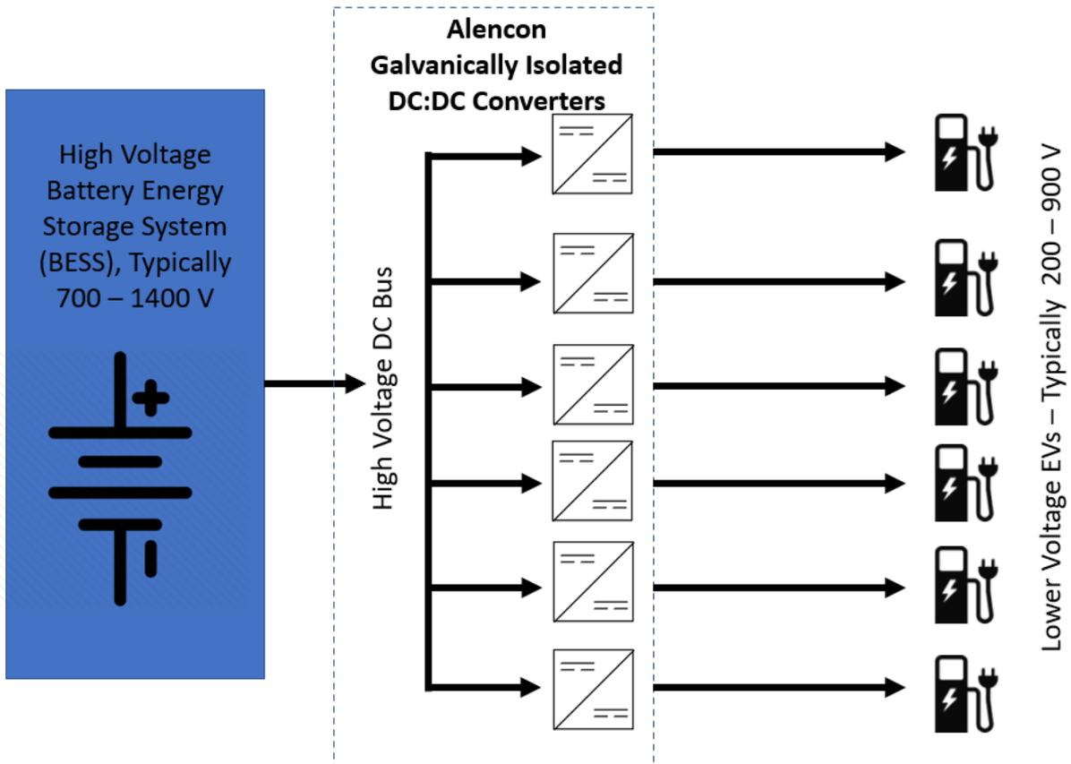
Figure 2 The graphic above shows how Alencon’s galvanically isolated DC:DC converters can provide the lynch pin between a large, higher voltage battery energy storage systems and lower voltage PEV’s being charged from it. The graphic above shows unidirectional charge from a BESS to an EV. Alencon devices also allow for bi-directional charge, which can facilitate vehicle to grid charging (V2G).
