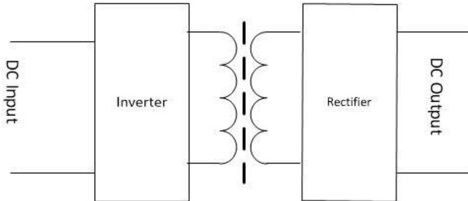
*Figure 3 Alencon’s DC:DC converters achieve galvanic isolation through the placement of a unique, high frequency transformer between the input and the output. This isolation allows EVs to be charged from larger BESS safely through contactless means while providing myriad of other benefits. This approach also makes it easier to handle large voltage differences between the BESS and the vehicle.*
