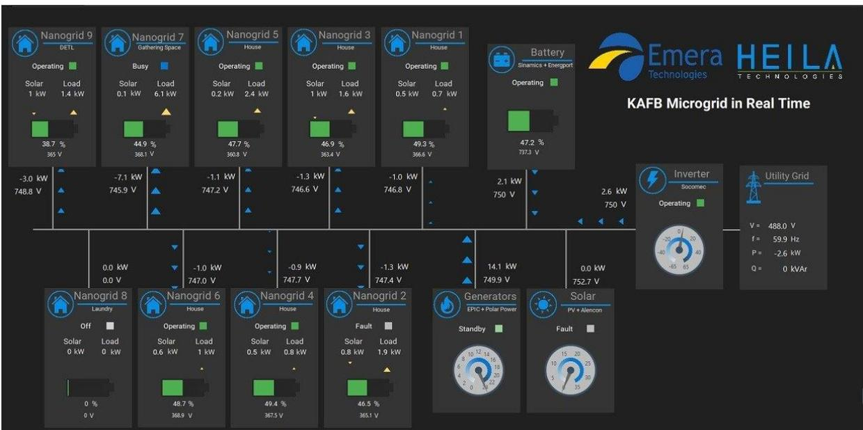
Figure 2: The Emera Microgrid provides real time monitoring and control of all the loads and energy sources to which it is connected.
