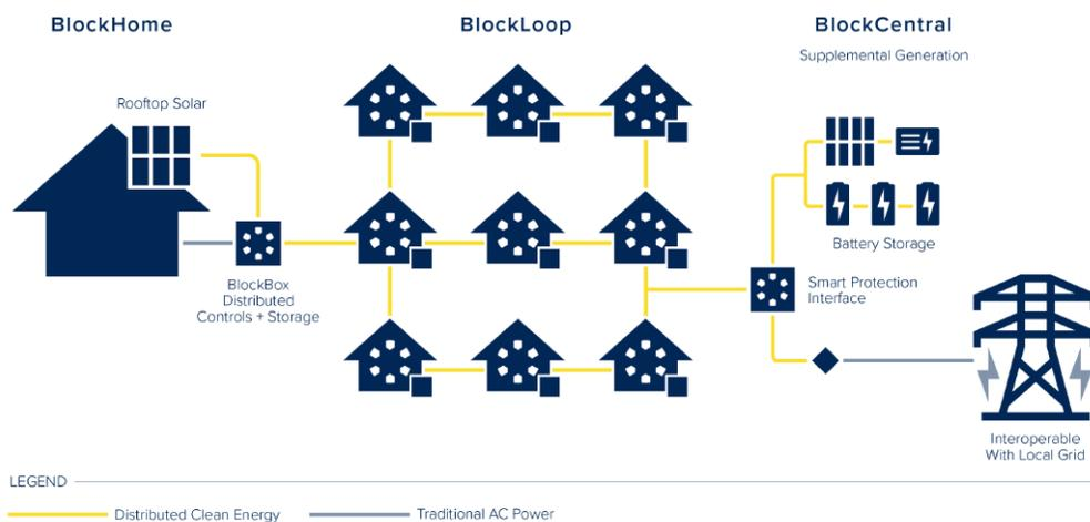
Figure 1 Emera’s BlockEnergy™ Smart Platform Microgrid topology is shown above. In the Emera “hybrid” Microgrid, a central DC coupled solar and battery storage system is connected to the grid and clean energy is distributed to individual loads via a DC distribution system. Each load (node) in the nano-grid has its own localized generation and storage infrastructure as well.
